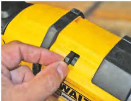
▲ This switch resets the driving blade if the gun stalls when a jam occurs
